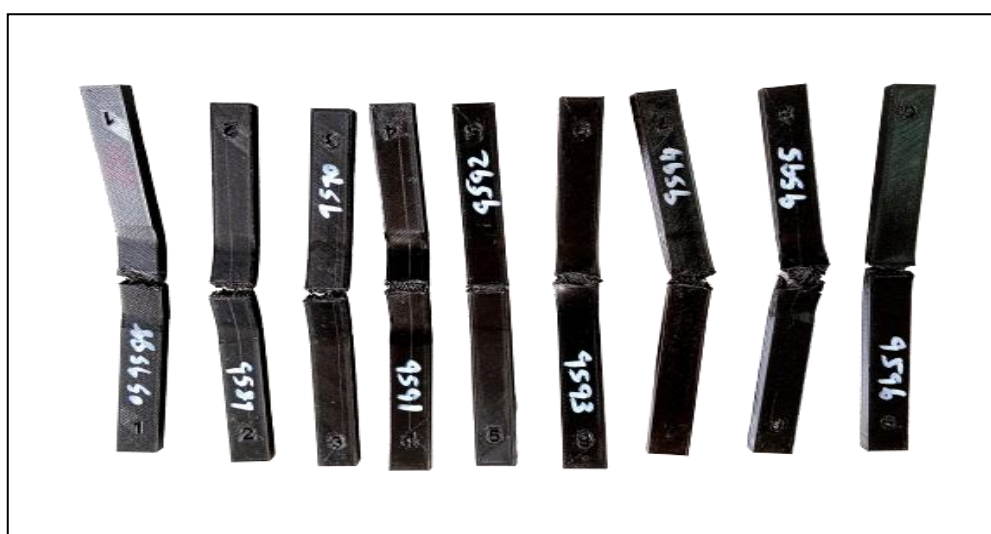
Figure 4. Fractured FDM printed PET-G Specimens - three - point bending test
